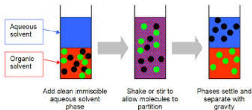
Figure 2. A schematic diagram of solvent extraction process
